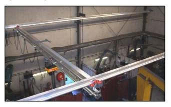
A gantry crane can be mounted from the roof or freestanding. Freestanding gantry cranes can also be created to be mobile, although they are generally designed to cover the entire workspace so that mobility is not an issue.
